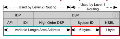
Any number (usually 49 indicating Private IS-IS) Area (16 bits): System ID (48 bits): MAC Address of any interface of this Router NSEL (last 8 bits): Zero (NSEL = 00 means the device itself. The NSAP with a NSEL = 00 is known as a NET) e.g. AFI.Area . System ID(MAC) . NSEL (always 00 on ISs) 49.0001.2222.2222.200
